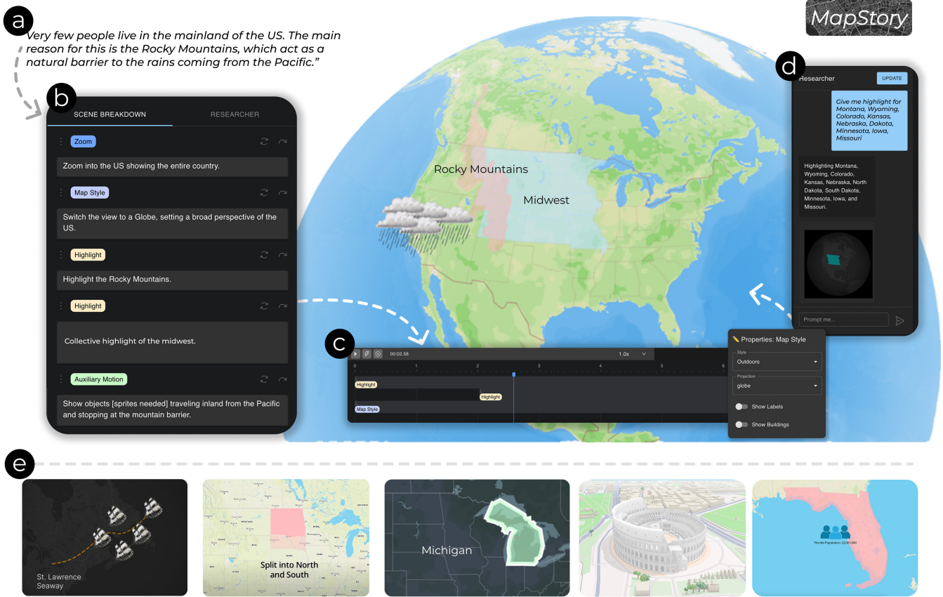
Figure 1: MapStory is an LLM-powered tool for prototyping map-centric animations from natural language scripts. Users write and edit a script (a), which generates an editable scene breakdown (b). The animation is shown on a timeline with a properties panel (c), and a researcher module retrieves and updates geospatial data (d). We showcase various map animation examples (e).
